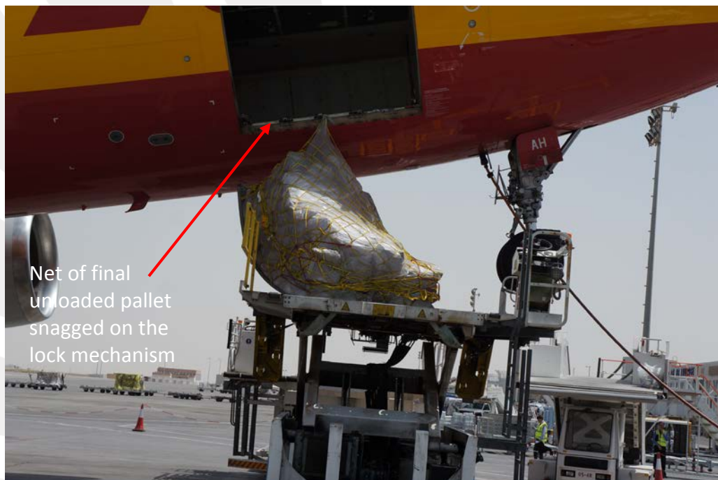
Figure 11. Net of the unloaded final pallet snagged on the lock mechanism of forward cargo hold door.
